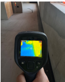
Thermal imaging camera inspection
