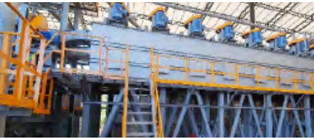
Acid leaching tank for decomposition of contaminants
