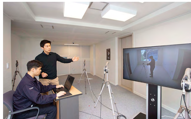
Inter-floor noise assessment at H Silent Lab
