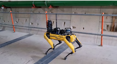
Inspection of TBM tunnel site using robotics
